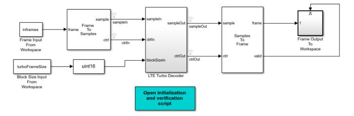
The **LTE Turbo Decoder** subsystem consists of the LTE Turbo Decoder block. This block is set to run for a frame size of 6144 systematic bits and 6 iterations of decoding.
