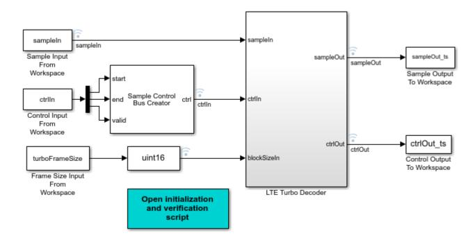
The **LTE Turbo Decoder** subsystem consists of the LTE Turbo Decoder block. This block is set to run 6 iterations of decoding.
